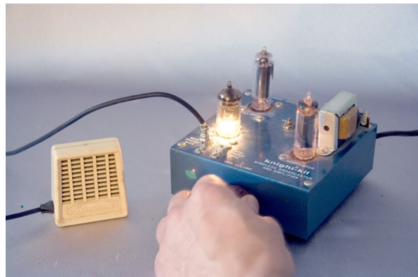
Broadcaster turn-on: Current surges through the 12AX7 tube as the Broadcaster is turned on for the first time. (Courtesy: Author)
